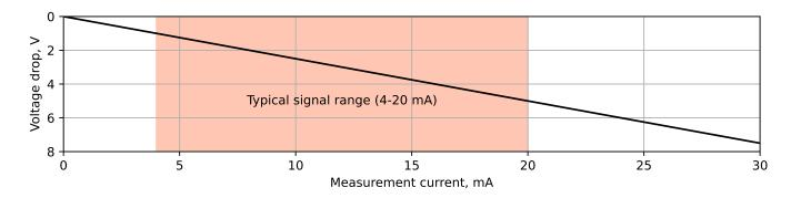
Please consult the documentation of the external 4-20 mA signal source to verify that a load of  $250 \Omega$  and the associated voltage drop are applicable to the particular device. Failure to observe these constraints might result in unstable operation or damage to the 4-20 mA signal source device.
